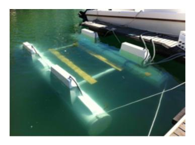
2. Attach the hose pipes to the "UP" hose connectors on the Blower House (top four connectors)
